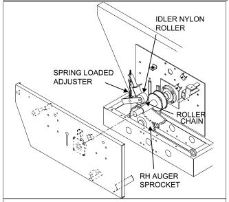
The RH auger chain drive, figure 10, is automatically tensioned by a spring loaded idler nylon roller. The extension spring should extend 3/4" from its neutral 4" total length.
