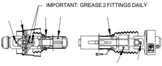
jack shaft reduction sprocket weldments, and the third auger drive shaft on the front drive. The zerks are accessible by the right front side grease bank and through the access holes in front plate. Be careful not to over grease.
