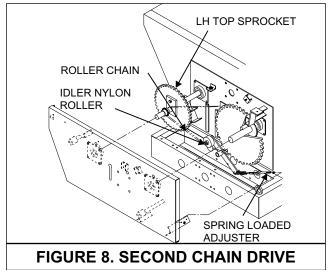
The second chain drive (large RH top sprocket to the large LH top sprocket, figure 8) is automatically tensioned by a spring loaded idler nylon roller. The extension spring should extend 2" from its neutral 5" total length.
