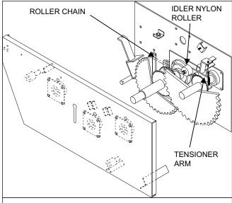
The third chain drive is automatically tensioned by a spring-loaded nylon idler roller. The extension spring should extend 3/4" from its neutral 4" total length. See figure 9.
