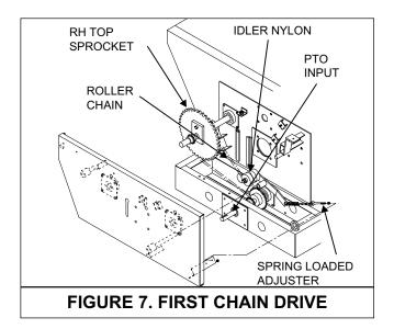
The first chain drive (PTO input shaft to the large RH top sprocket, figure 7) is automatically tensioned by a spring loaded idler nylon roller. The extension spring should extend <u>2</u>" from its neutral 5" total length.
