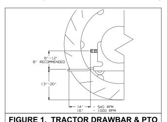
to the standard 16" drawbar & PTO relationship will ensure that the PTO drive shaft will not become over-extended.
