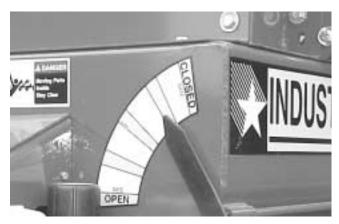
FIGURE 4. FLOW CONTROL GATE INDICATOR
