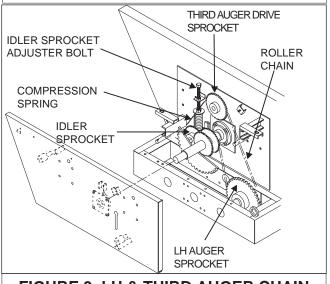
FIGURE 9. LH & THIRD AUGER CHAIN DRIVE
