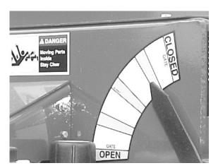
FIGURE 4. FLOW CONTROL GATE INDICATOR
