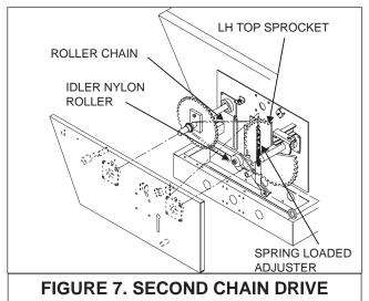
The second chain drive (large RH top sprocket to the large LH top sprocket, figure 7) is automatically tensioned by a spring loaded idler nylon roller. The extension spring should extend <u>2</u>" from its neutral 5" total length.
