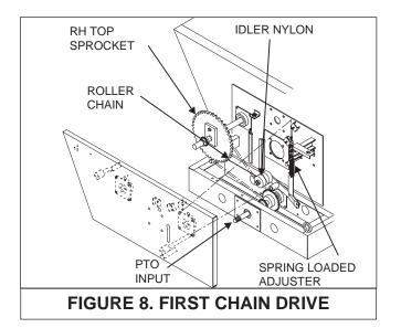
The first chain drive (PTO input shaft to the large RH top sprocket, figure 8) is automatically tensioned by a spring loaded idler nylon roller. The extension spring should extend 2" from its neutral 5" total length.
