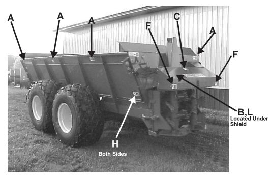
ACAUTION: READ ALL DECALS ON THE SPREADER AND IN THIS MANUAL. KEEP THESE DECALS CLEAN AND REPLACE ANY LOST OR DESTROYED DECALS. BECOME FAMILIAR WITH ALL TRACTOR AND SPREADER CONTROLS.
