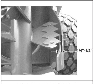
FIGURE 12. MATERIAL GUIDE CLEARANCE
