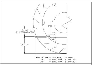
FIGURE 1. TRACTOR DRAWBAR & PTO SPECIFICATION
