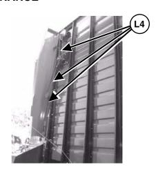
Clean out all forage material from inside the box, roof, and on the outside of the box. Clean the front cross apron on the top and in the lower pan (chain return) area. Clean out the deflector shield at the rear of the box, both inside and outside.
