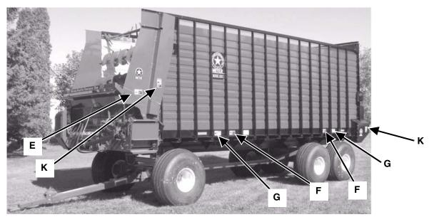
CAUTION: READ ALL DECALS ON THE FORAGE BOX AND IN THIS MANUAL. KEEP THESE DECALS CLEAN AND REPLACE ANY LOST OR DESTROYED DECALS. BECOME FAMILIAR WITH ALL TRACTOR AND FORAGE BOX CONTROLS.
