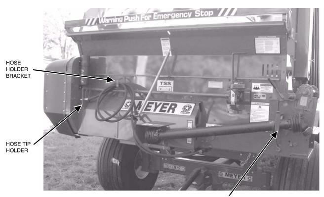
IMPORTANT: Support hoses on Hose Holder Bracket to relieve weight & stress from hose tip holder.
