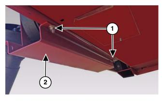
5. Remove the two bolts (Item 1) for the PTO shaft cover (Item 2).
