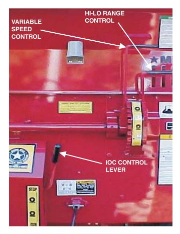
Three levers control operating the front unloading unit of the forage box.
