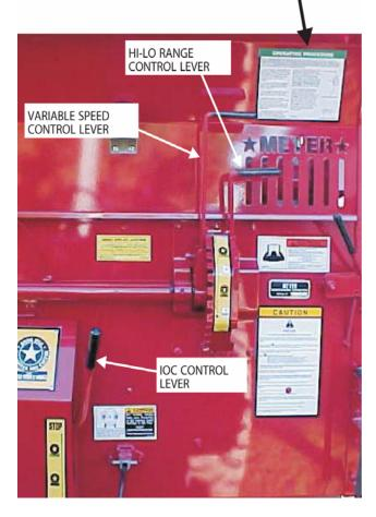
Three levers control operating the front unloading unit of the forage box.
