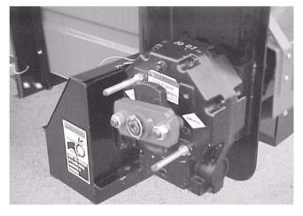
(Shield Removed For Illustration Purposes Only) **COUPLING PLATE**
