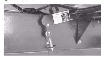
**PRIOR TO 08 SERIAL NUMBERS** - To tighten the main aprons, tighten down the anchoring eye bolts centrally located at each side of the forage box on the steel 10" stringers.
