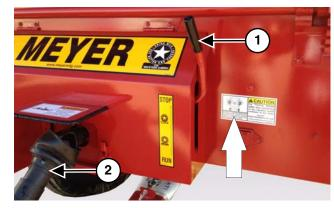
3. Release the two latches (Item 1) and raise the front chain shield assembly (Item 2).
