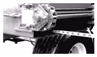
Correct adjustment of the cross apron chain occurs when 12" of chain, APRON SLAT does not touch the BOTTOM PAN of the cross apron return area at the discharge opening. To tighten the chain, loosen the two bolts securing the slotted bearing bracket at each side of the discharge opening. Tighten the chain by tightening the nut on the adjuster bolt. Adjust both sides equally. Retighten the bearing bracket bolts.
