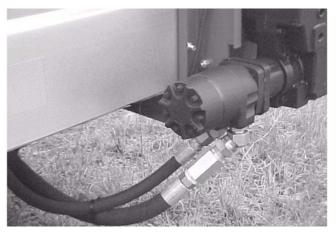
**HYDRAULIC CHECK VALVE AT REAR OF BOX**
