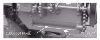
Remove clean-out panel on a regular basis to clean out accumulation of foreign material build-up. Keep this area clean for proper cross conveyor chain operation.
