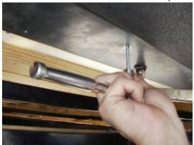
for the other side. Tighten your main apron chain to the appropriate tension. See your 4200 Owner's Manual in the Adjustments Section for proper chain tightening, or go to our website at www.meyermfg.com and look for your model on the Manual page.
