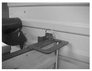
When the False Front Gate and mounting brackets have been removed, replace the 3/8" bolts to fill the holes.
