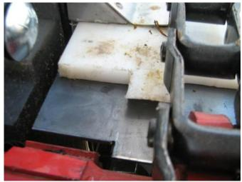
bump up to the bottom of the poly floor, and stick out towards the drive shaft. In the picture to the right, notice the left formed piece underneath the poly floor. The picture below shows a view of the left end of the left apron floor seal from underneath the box. Repeat the above step to insert the right apron floor seal underneath the poly floor.
