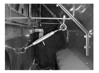
Hook turnbuckle as shown and draw up tight. Turnbuckle will hold center of door up tight to the grain kit.
