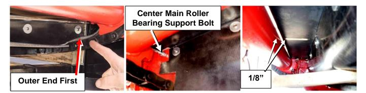
Insert the side toward the outside of the box first. Next slide the side toward the center in lifting up and around the center main roller bearing support bracket bolt. Then slide the whole assembly back toward the main roller so that there is a 1/8" gap between the main roller and the seal kit plate. Clamp to hold in place.
