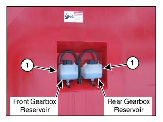
Check the 2-speed gearbox oil level daily to prevent abnormal component wear. Add new oil to the reservoir tank (Item 2) if the oil level is not at the oil reservoir mark.
