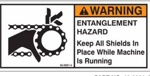
PART NO. 46-0001-4 (Located on top of shield)
