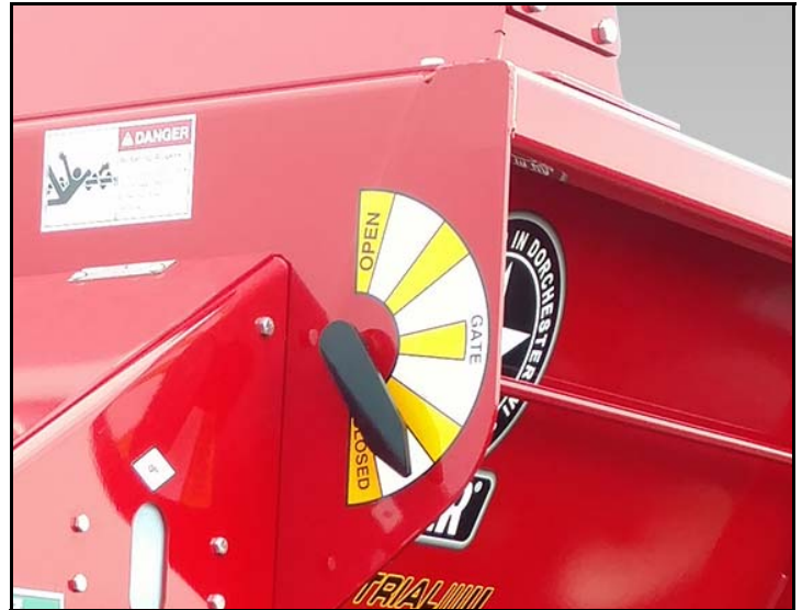
FLOW CONTROL GATE INDICATOR
