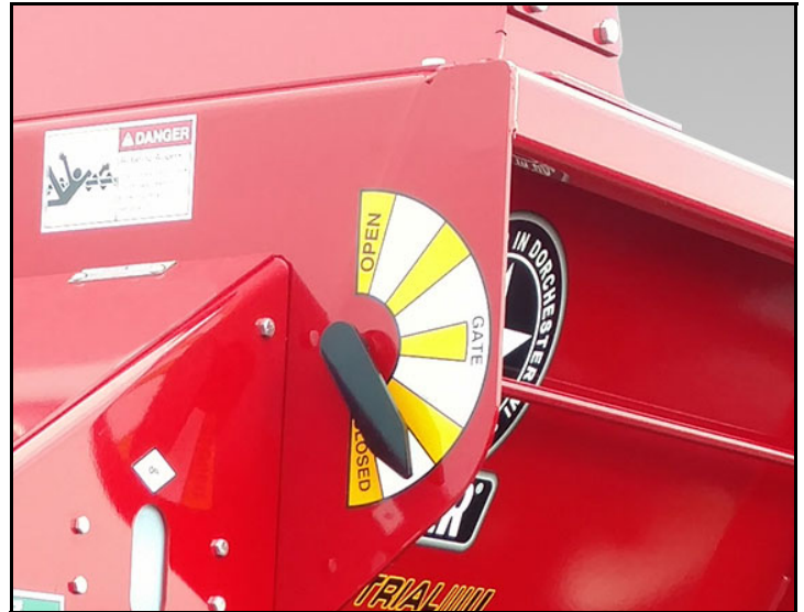
FLOW CONTROL GATE INDICATOR
