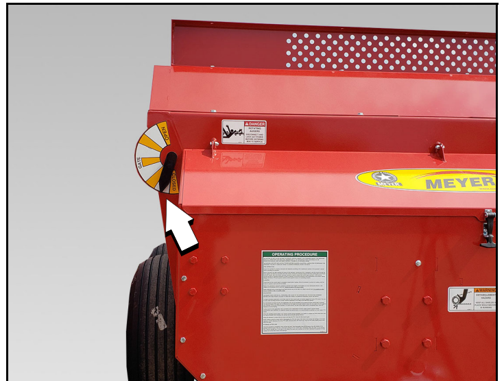
SXR500 FLOW CONTROL GATE INDICATOR
