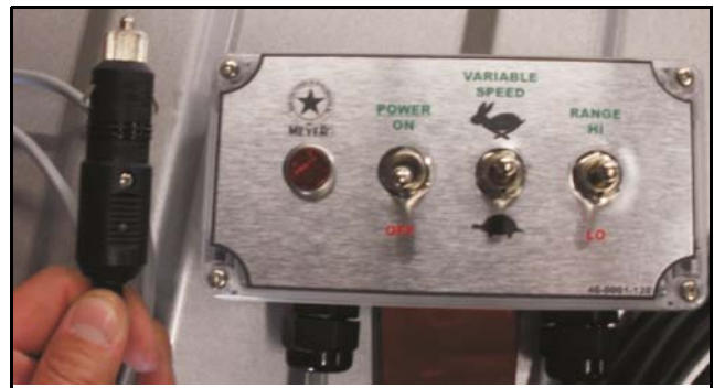
Figure 2. Controller Power Cable
