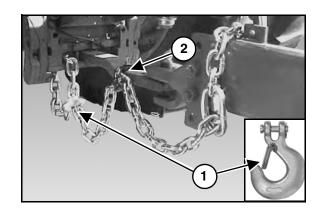
NOTE: Do not use the intermediate support (Item 2) as the attaching point.
