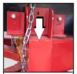
Prior to 2016 Model Year Tandem Axle Serial Number Plate EXAMPLE: 1514201
