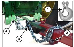
The chain must be of adequate size to hold the weight of the loaded wagon.
