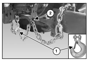
The chain must be of adequate size to hold the weight of the loaded trailer.
