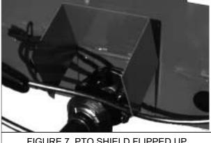
FIGURE 7. PTO SHIELD FLIPPED UP
