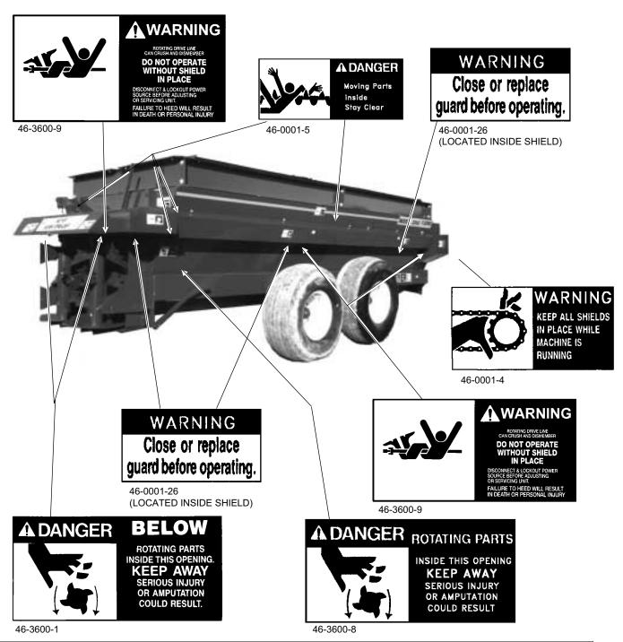
READ ALL DECALS ON THE SPREADER AND IN THIS MANUAL. KEEP THESE DECALS CLEAN AND REPLACE ANY LOST OR DESTROYED DECALS. BECOME FAMILIAR WITH ALL TRACTOR AND SREADER CONTROLS.
