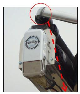
NOTE: The brake circuit prevents the brake from being completely removed from the assembly. It is OK to leave the brake motor hanging from the wire leads.
