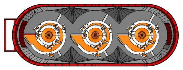
With the NEW F3 Vertical Triple Auger Mixer comes a new design! The 93" augers overlap each other by 6" for Superior mixing in the Triple Auger Market! Along with this design comes superior feed transfer from auger to auger!
