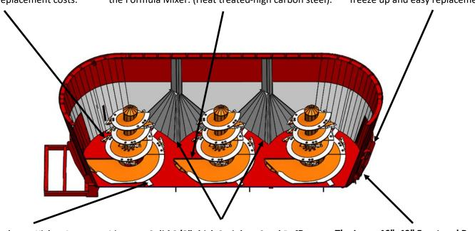
**Dual Auger Discharge Kicker Arms** provide 2 extra sweeps with every auger revolution, allowing smoother feedout in less time. **Solid 3/8" thick Stainless-Steel Baffles** are Standard Equipment making them nearly a lifetime baffle.
