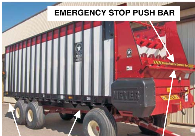
EMERGENCY STOP TRIP CABLES EXTENDING ALONG BOTH SIDES
