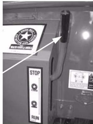
INDEPENDENT OUTFEED CLUTCH CONTROL LEVER
