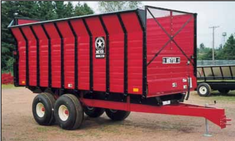
18' trailer mount with flared side. (Hydraulic Drive Recommended)
